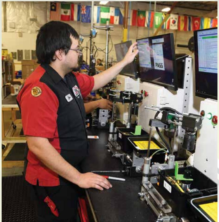
Maintenance Technician John Torres verifies testing criteria of the PSI manifold. Testing is a crucial step in production as all PSI and TST products are safety related.
