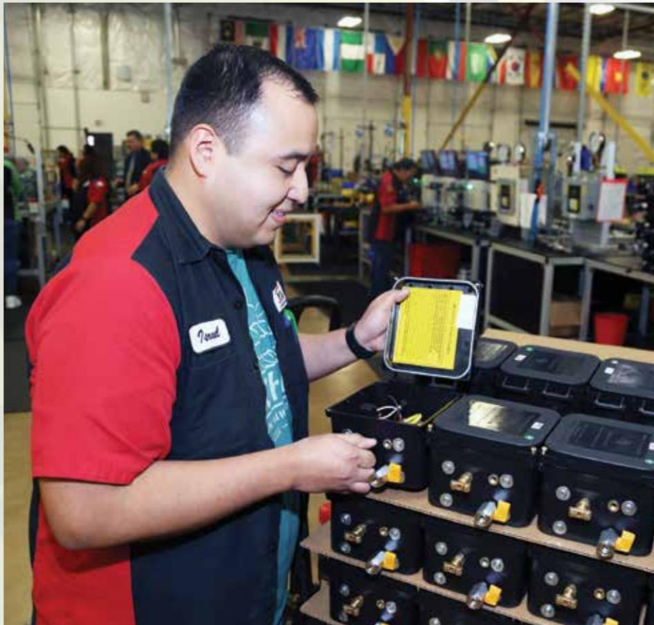
Israel Perez performs a 16-point qualification of control boxes following a final test. All assembled products are tested under the control of a team cell leader before they are forwarded to quality control for inspection.
